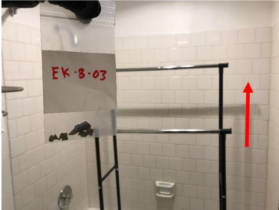
HA No. 8. 4"x 4" white ceramic tile, white grout, yellow mastic, and white joint compound (M)
