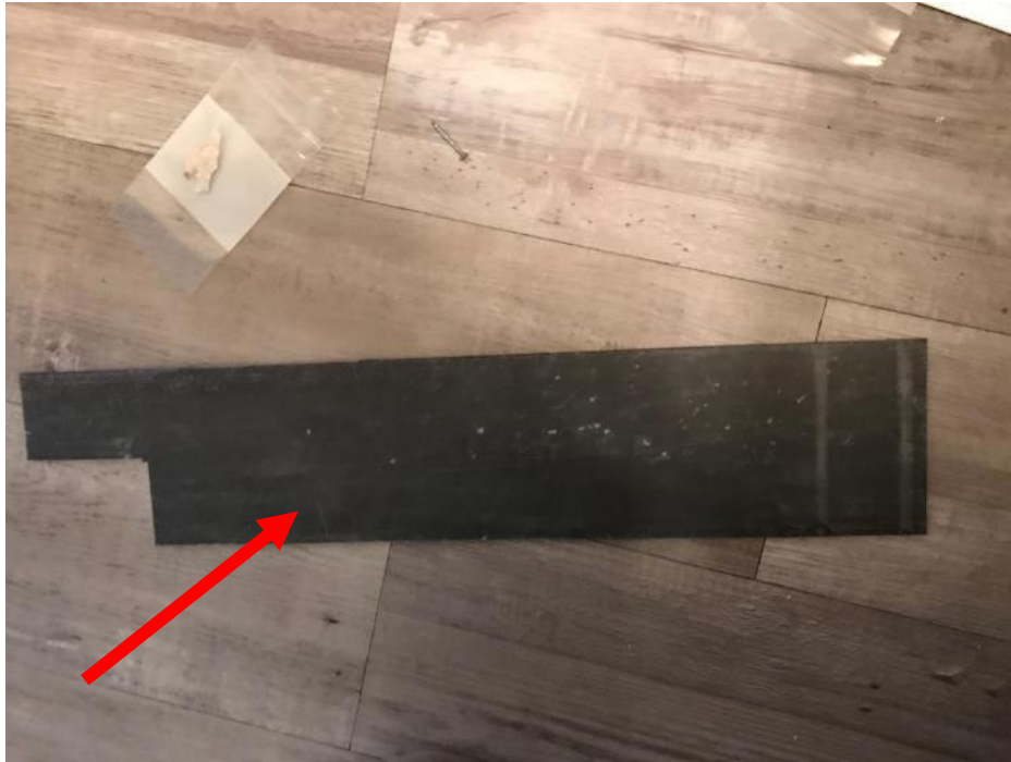
HA No. 2. Grey wood pattern tongue and groove vinyl floor tiles and grey leveling compound (M)
